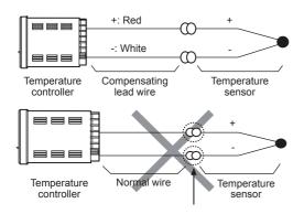
a connecting point becomes a temperature sensor, that generate an error.
