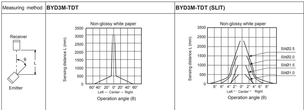
※Above characteristic is from 400mm sensing distance to install transmitted beam type slit (Ø1, Ø1.5, Ø2, Ø2.5).
