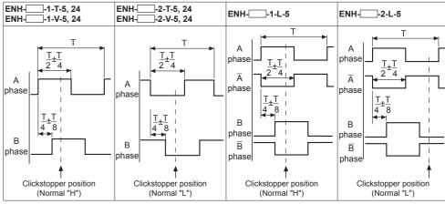
\*\*Clickstopper position Normal "H" or Normal "L": It shows the waveform when the handle is stopped.
