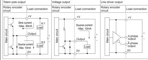
\*\*The output circuits for A, B phase (line driver output is A, A, B, B phase) are same. \*\*Totem pole output can be used for NPN open collector type (\*\*1) or voltage output type (\*\*2).
