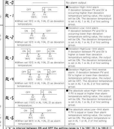
% "b" is interval between ON and OFF the setting range is 1 to 100 % (0.1 to 100.0 % ) and can be set at "RHYS" mode in first setting group.
