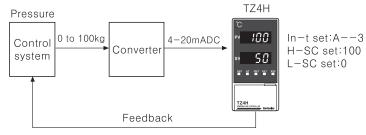
\*In case of using the converter mode, please select the inner switching pin according to the chart in "Selection switch for Input sensor/Voltage/Current".
