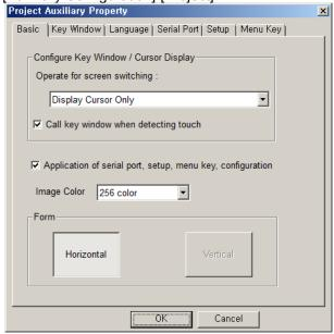
2nd At [Serial Port] tab, set CH1 port configuration.
