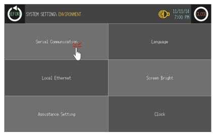
3rd CH2 protocol is set as CT6M-2P as PLC type from GP Editor but downloaded CT6M-2P protocol is not applied directly. (Communicates with EDITOR from CH2). Touch protocol display item of CH2 to set CT6M-2P.
