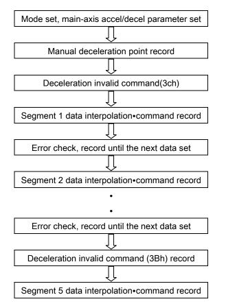
Be sure that manual deceleration point is the value for the number of main axis basic pulses from node 5. For example, deceleration pulse is used 2000, the number of basic pulses which is ouput to node 5 is 5000. Set manual deceleration point as 5000-2000=3000. From starting deceleration to stopping, it must be set in one node.
