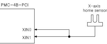
As the above table, set signal logic level of Step1 and Step2 as search direction as same. (It is possible to set logic level as reverse.) When home searching at Step1 with high speed and home signal becomes active, it stops by deceleration.
