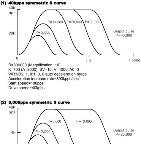
2.0 4.0sec R=8000000 (Magnification: 1) K=2000 (A=8000), SV=10, V=8000, A0=0 WR3/D2, 1, 0:1, 0, 0 auto deceleration mode Acceleration increase rate=31kpps/sec<sup>2</sup> Start speed=10pps Drive speed=8000kpps
