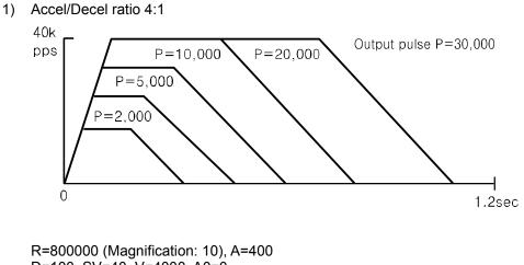
R=800000 (Magnification: 10), A=400 D=100, SV=40, V=4000, A0=0 WR3/D2, 1, 0:0, 1, 0 auto deceleration mode 60H/WR6/D3:1 triangle form prevention ON Acceleration=500kpps/sec Deceleration =125kpps/sec Start speed=400pps Drive speed=40kpps
