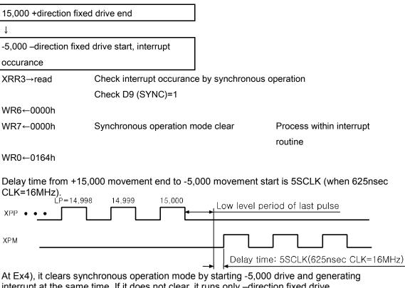
At Ex4), it clears synchronous operation mode by starting -5,000 drive and generating interrupt at the same time. If it does not clear, it runs only –direction fixed drive. When drive stops by +direction limit(LMT+) or emergency stop(EMG) during +15,000, the next -5,000 drive runs. If this situation may be the system problem, be careful that synchronous operation use.
