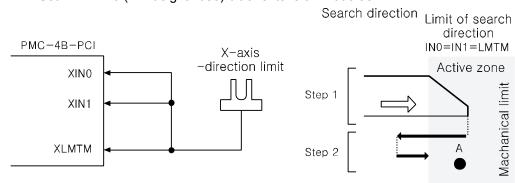
Set WR7/D10 (Limit signal use) bit of extension mode as '1'.
