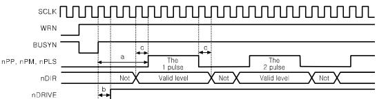
a. In interpolation drive, drive pulse (nPP, nPM, nPLS), it outputs the 1 pulse after SCLK4 cycle at ↑ of BUSYN.
