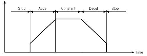
In each axis drive, the acceleration/constant speed/deceleration status of drive speed outputs at D2(ASND), D3(CNST), D4(DSND) bit of RR1 register for each axis and at nOUT6/ASND, nOUT7/DSND signal. Because signal output is used with general output signal terminal, to output drive status, set D7(OUTSL) bit of WR3 register as '1'.
