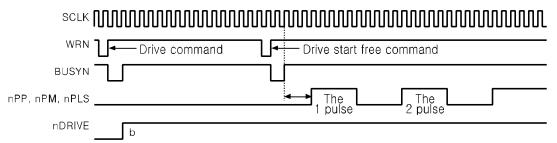
a. After drive pulse(nPP, nPM, nPLS) of each axis cycles to SCLK3 at  $\uparrow$  of BUSYN for drive start free command write, the 1-pulse is output at the same time.
