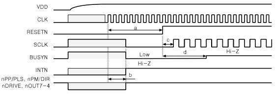
a. Reset input signal RESETN requires low level over CLK×4 cycel after CLK inputing.
