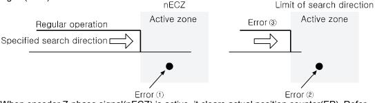
When encoder Z-phase signal(nECZ) is active, it clears actual position counter(EP). Refer to the Actual position counter clear by external signal '5.3.4 Actual position counter clear by external signal'.
