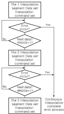
In consecutive interpolation, use D9(CNEXT) bit of RR0 register. This bit is the data of the next interpolation node and it is the whether to set interpolation drive command during interpolation drive during interpolation drive. '1' means set available and '0' means set unavailable.
