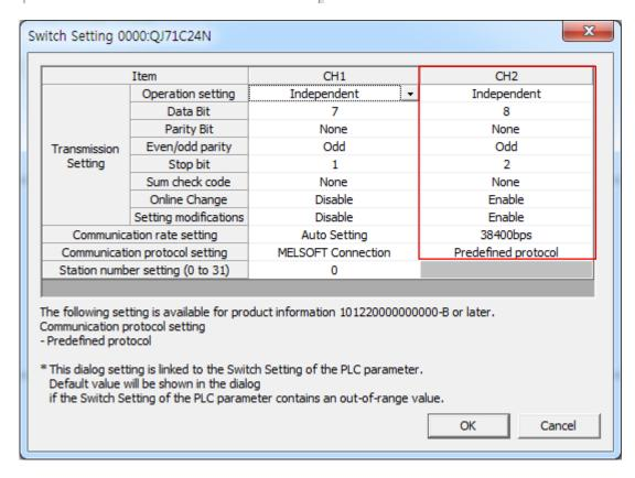
2nd Run [Tool - intelligent Function Module Tool – Serial Communication Module – Predefined Protocol Support Function] on menu.
