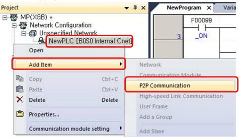
4th You can check the added P2P setting window below standard network. Doulble-click NewPLC[B0S0 Internal Cnet] and [Standard Settings – Cnet] dialog box is available.
