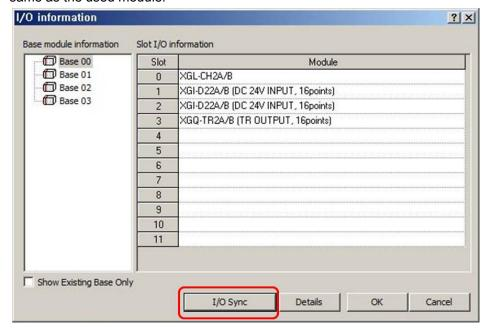
5th When I/Osyncronizing is completed, the used communication module is added at the below standard network. Double-click the right communication module.
