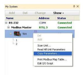
4th Right-click the unit which parameters are saved and select 'Parameter Select'. The parameter values of the unit is loaded at the right side of the dialog.
