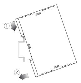
2nd Engage the top and bottom rail locks. Push until it clicks and the rail locks firmly fix the DIN rail.
