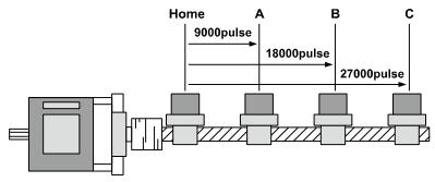
Relative position movement sets a distance to drive from present coordinates. This is INC, LID, CID, FID, or RID command in program mode, and preset mode of [Manual] tap.
