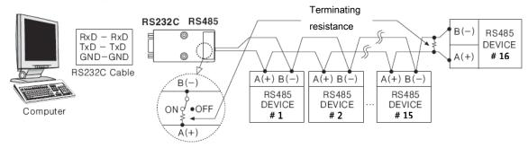
(The connected communication converter is SCM-38I of Autonics.)
