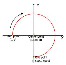
In the above image, center coordinates (5000, 0) and end coordinates (5000, -5000) are set from present coordinates (0, 0) using FID command. The radius of the circle is 5000, and it drives from present coordinates (0, 0) to end coordinates (5000, -5000) in CW direction.
