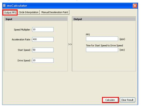
Select [Output PPS] tab and enter speed multiplier, acceleration rate, initial speed, and drive speed in [Input] field on the left side, and click [Calculate]. The PPS of output and time for start speed to drive speed is shown in [Output] field.
