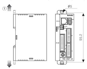
2nd Insert bolts and tighten them. (with tightening torque of 0.5N•m to 0.9 N•m.)
