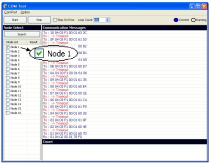
4th Set [Loop Count] to 5 and click [Start] to start the test. After 5 Cycle, a confirm dialog box is open and notifies you that the test is complete. Click [OK] to close the box. [Result] box in [Node Select] section displays the test result as OK.
