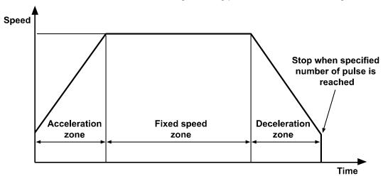
Speed multiplier, initial speed, drive speed, and acceleration rate must be set in [Parameter] to run fixed pulse acceleration/deceleration drive. For asymmetry acceleration/deceleration drive, it is needed to select [Decel] for [Deceleration Value] in [Operation Mode] and then set the deceleration rate separately.
