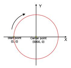
The above image shows the motion of CID command with the radius set to 5000 from the present position (0, 0). The radius of the circle is 5000, and it drives from present coordinates (0, 0) to center coordinates (5000, 0) in CW direction. Radius range is -8,388,608 to +8,388,607.
