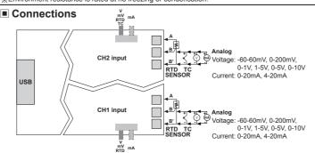
XInput parts and USB cable connection part are insulated each other
