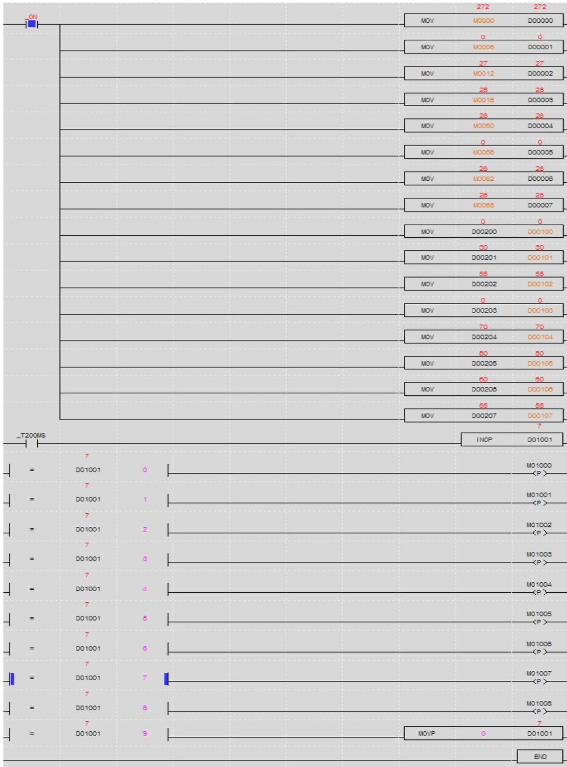
D00000 to D00003 are present temperature values of CH1 to CH4 at station 1.
