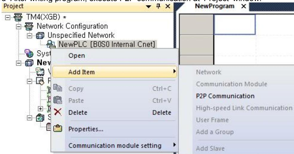
4th You can check the added P2P setting window below standard network. Double-click NewPLC[B0S0 Internal Cnet] and [Standard Settings – Cnet] dialog box is available.
