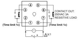
%1: AC/DC voltage: 100-240VAC 50/60Hz, 24-240VDC 24VAC 50/60Hz, 24VDC
