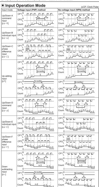
XA: over min. signal width, B: over than 1/2 of min. signal width If the signal is smaller than these width, it may cause counting error (±1). \*\*The above specifications are subject to change and some models may be discontinued
