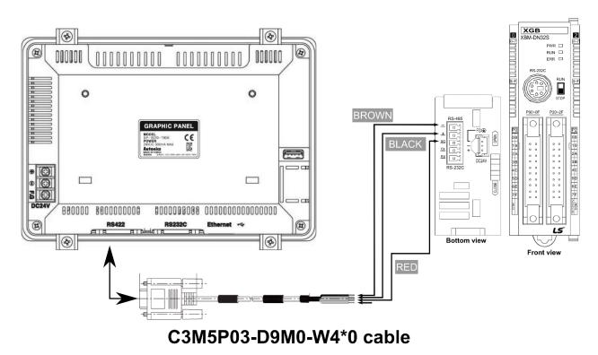
Communication cable pin details and dimensions 1.4 (Autonics model: C3M5P03-D9M0-W4\*0)
