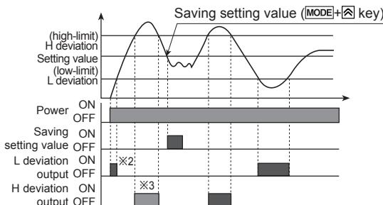
※2: When selecting initial comparative output limit function, it does not transmit outputs.
