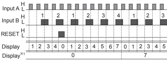
※1: When the display cycle[d1 5PL] setting is OFF, it will maintain the quantity of input A until the value of input B reaches the setting value B[Coun.b].
