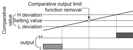
※After supplying power, there is no comparative output of L deviation (■).
