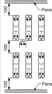
※Screw tightening torque for mounting: 1.8 to 2.5N·m
