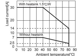
⚠ Please supply less than 50% of the rated load current when installing several SSRs closely due to decreasing effectiveness of protection against heat.
