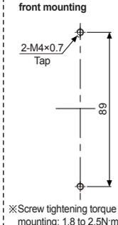
○ Installation interval (unit: mm)
