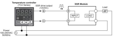
When selecting cycle or phase control mode, the power supply for load and temperature controller must be the same.
