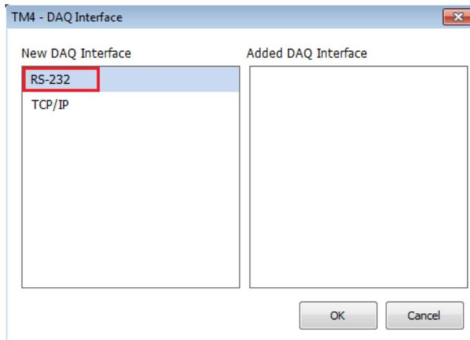
3rd Once the communication interface has been created, select this RS-232 interface in the 'My System' menu and set the PC communication port connected to the TM device. Then the different communication settings can be configure to match the TM device settings.
