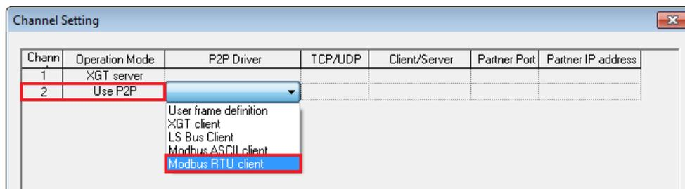
10th **The project has been properly set. Then you need to create your own 'P2P block' depending on the desired point in the TM device and your own PLC program and download the complete project to the XBC device by selecting [Online] – [Write], then clicking 'OK'.**
