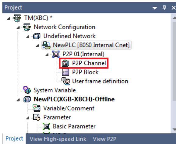
9th Set the 'P2P Driver' of the channel 2 to 'Modbus RTU client' and click 'OK'.
