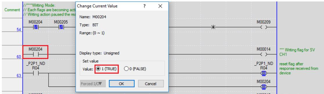
4th Using the same process, write the new CH2 SV value to the TM device (M0206).
