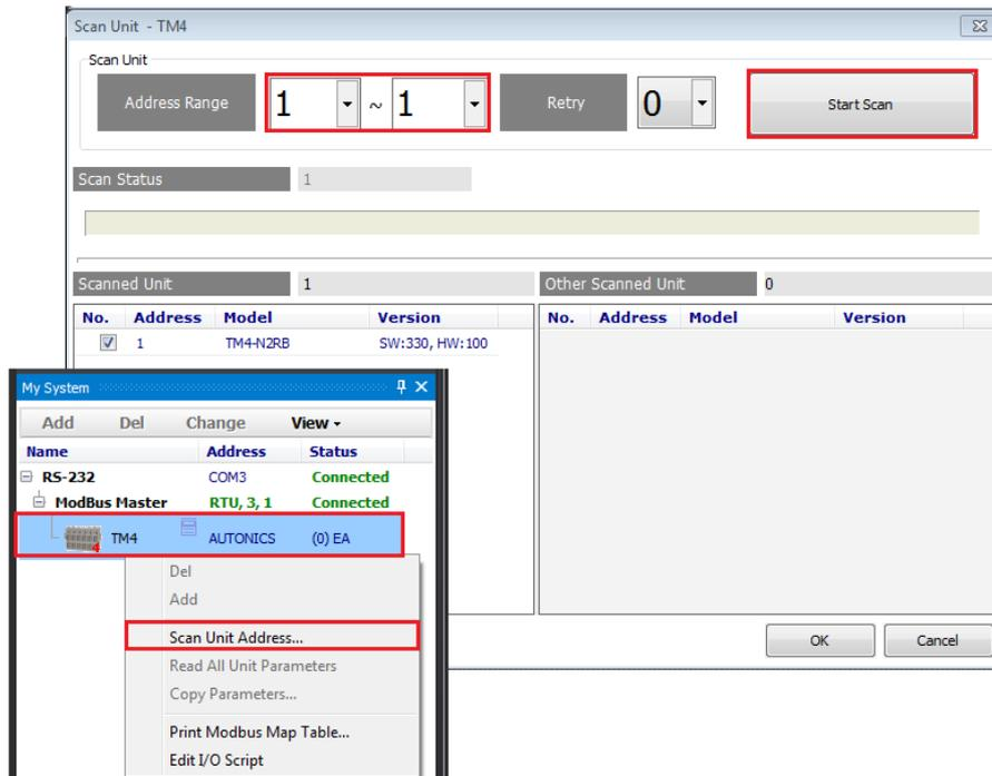
6th Your TM device has been added to the system list. To have access to its parameters, click right on the device in the 'My System' architecture and select 'Read All Parameters'.
