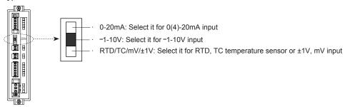
This unit is multi input product. Select the proper input with the input type selection switch and select this input type in  $! \ n^-P$  in program mode. The setting of input type selection switch and the input type  $! \ n^-P$  parameter should be same and it can display the proper measurement value. Factory default is 0-20mA.
