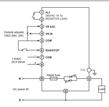
$\ensuremath{\mathbb{X}}\xspace \mathsf{R},$  S, U terminals are at the bottom of the unit. For wiring terminals, open the front cover.
