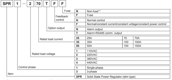
※1: Product is not equipped with a rapid fuse inside. Install the suitable fuse for rated load current of the model separately. (The performance of the product is guaranteed only when using the fuse provided by us.)
