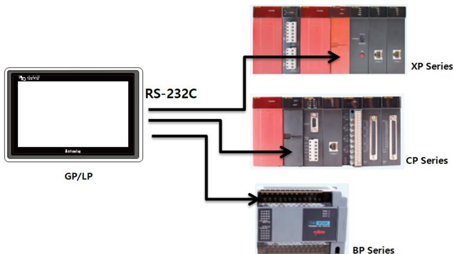
KDT CIMON BP/CP/XP Series CPU direct connection is connecting RS232C port of GP/LP and tool port (RS232C) of the PLC.
