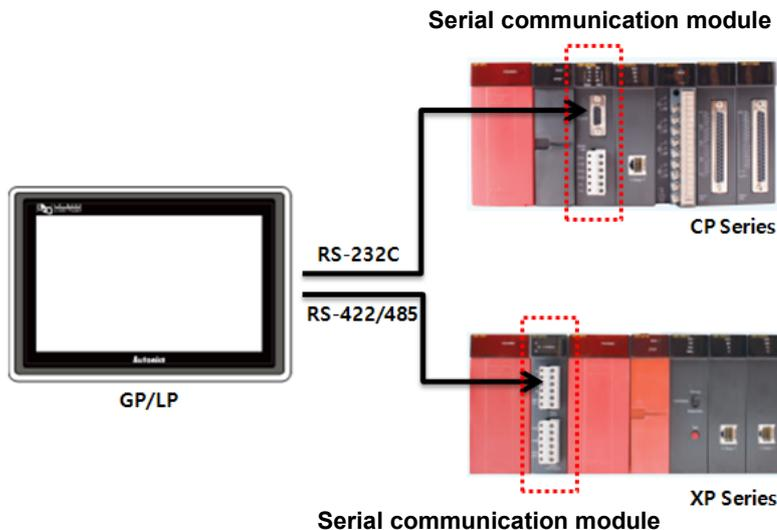
KDT CIMON CP/XP Series communication module connection is connecting RS232C, RS422/485 port of GP/LP and PLC compatible serial communication module (RS232C, RS422/485).
