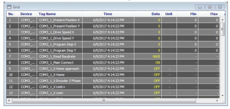
Grid column is editable. Right-click the head of grid, 'Select Column' dialog box appears. You can check the desired item to show.
