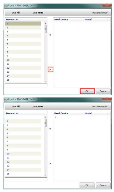
Now you can see the unit (address 1) under the device in My System. In case of adding same type of multiple devices, click [Add] button and add device. (Maximum 99 devices can be added.)
