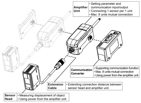
2nd Depending on user enviroment, connect RS485 or RS232C communication terminal to the PC which atDisplacement is installed.
