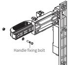
2. Tighten the hexagon nut+spring washer+inner lever with the designated tightening torque using a spanner with 10mm width. If the inner lever is screwed loosely, it may result in product failure.
