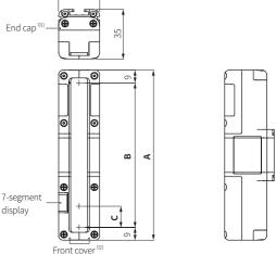
ving the end cap, there is the lamp output terminal (top) or the power supply terminal (bottom). ving the front cover, there is the setting switch (on the emitter and the receiver) or the PC communication
